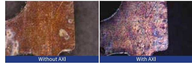
IC lead frame viewed at 210x magnification.
